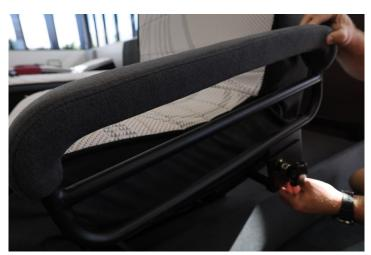
3. Locate the bolt as shown and fasten until as tight as possible.
